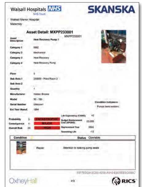
A record drawn from the new asset data showing the condition and likelihood of failure of a leaking pump.
