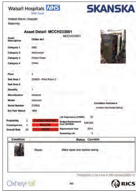
In all some 2,700 assets were surveyed - from distribution boards to air-handling units, generators, switch panels, boilers, chillers, pressurisation units, steam pipework, and medical gas plant.
